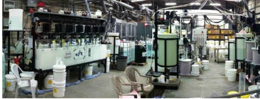
Figure 13.10 Pilot Plant (SX-Purification-Carbonation-Filtration-Washing Pulp)
