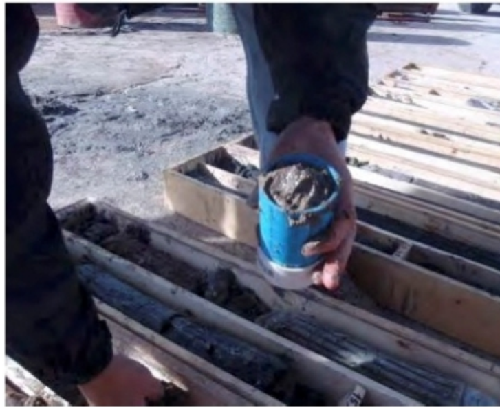
Figure 8.2 Collecting an Undisturbed Sample
