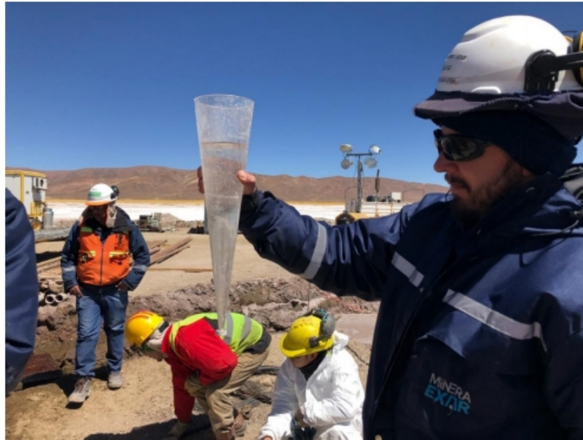
Figure 8.4 Measuring Sediment in an Imhoff Cone
