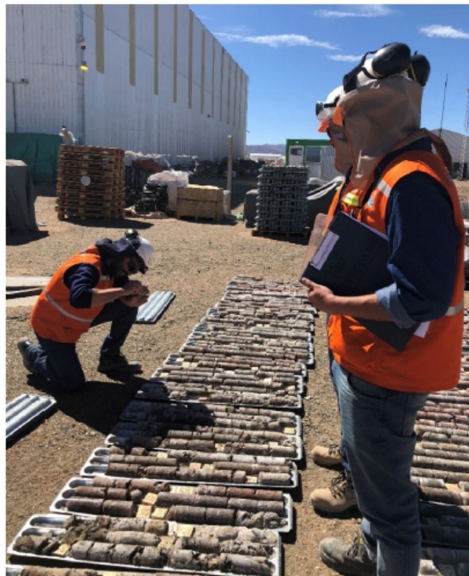
Figure 8.3 Collecting an Undisturbed Sample from Core
