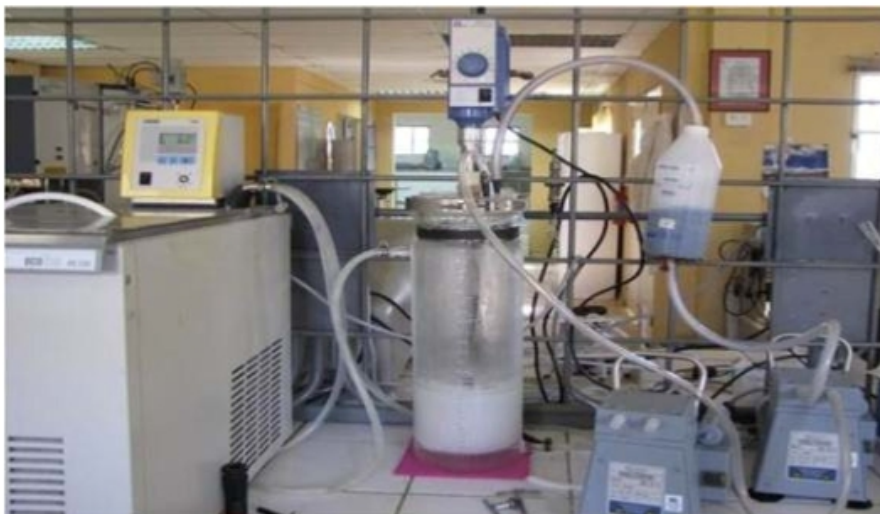
Figure 10.2 Dry Air Evaporation Tests
