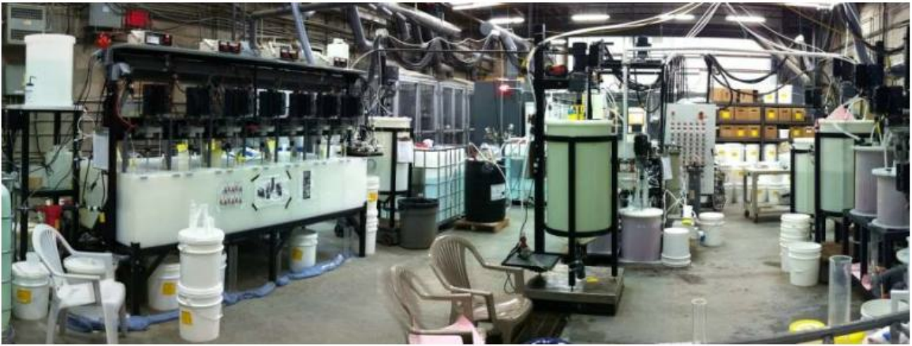
Figure 10.10 Pilot Plant (SX-Purification-Carbonation-Filtration-Washing Pulp)
