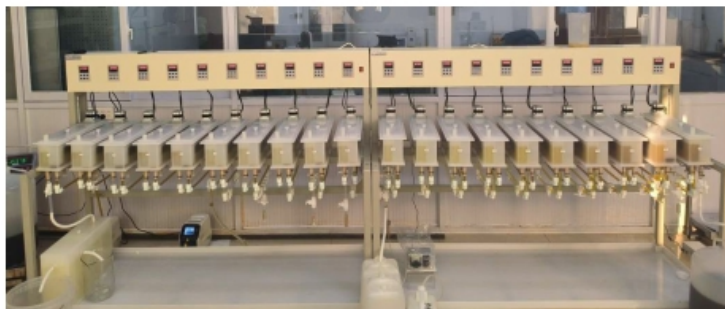
Figure 96: Continuous Extraction Device Diagram (Source: Ganfeng 2024)
