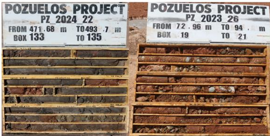
Figure 44: Lithologies from the HSUs Sandy (left photo) and Muddy (right photo) Alluvial and Colluvial Sediments (Source: Golder, Jan 2025)
