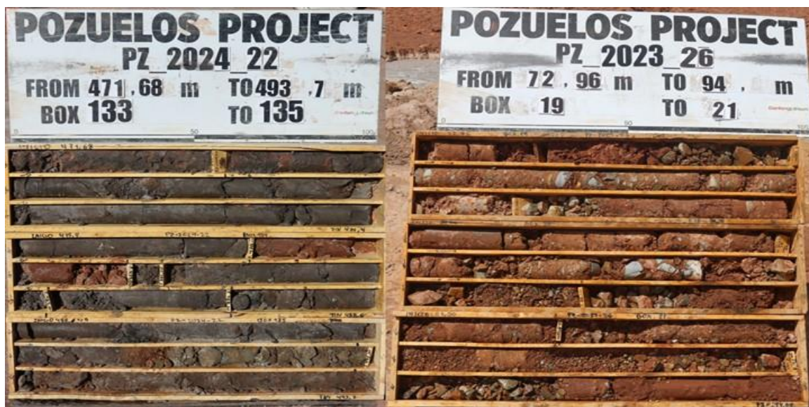
Figure 44: Lithologies from the HSUs Sandy (left photo) and Muddy (right photo) Alluvial and Colluvial Sediments (Source: WSP Golder, Jan 2025)
