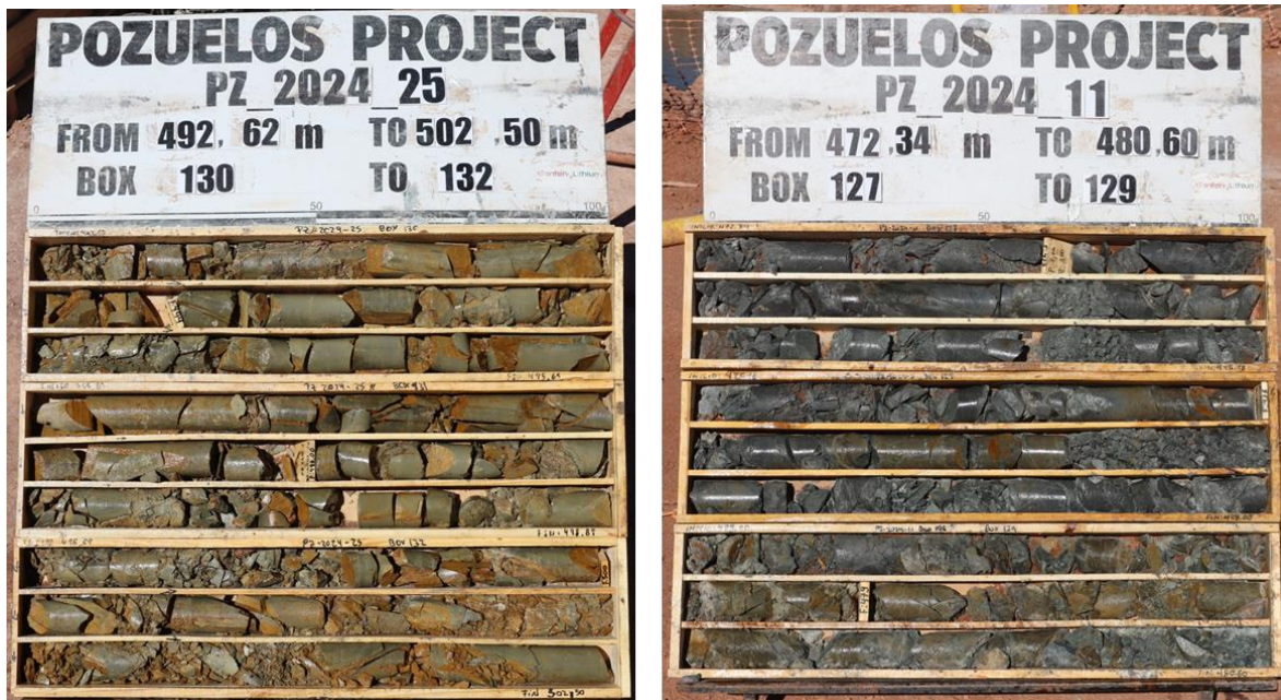
Figure 45: Lithologies of the HGU Fractured Aquifer (Source: WSP Golder, Jan 2025)
