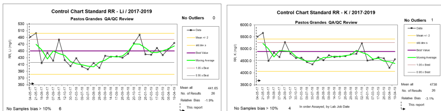
Figure 82: Graphical Analysis of Li (top) and K (bottom) within 'RR' Standards Assayed by SGS (Source: AW, Dec 2024)
