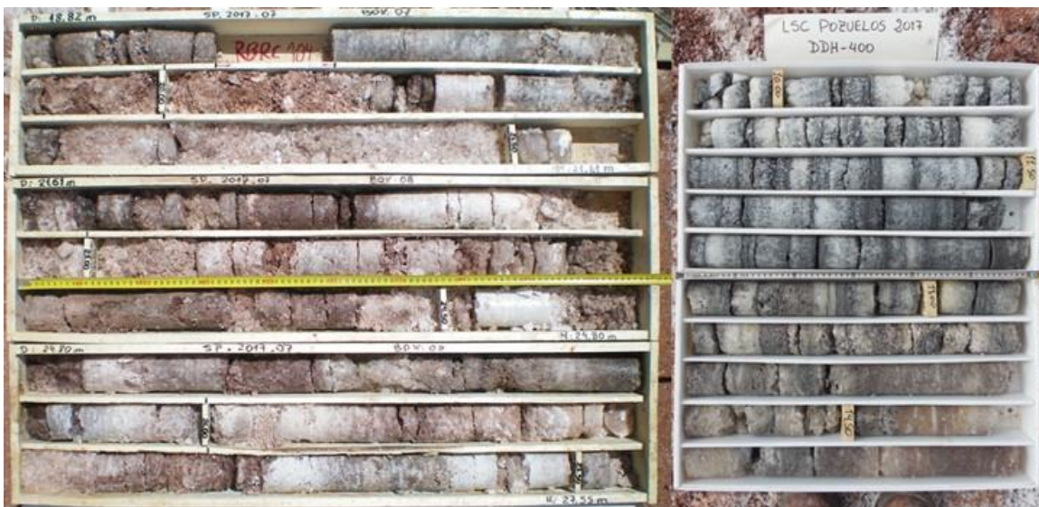
Figure 42: Lithologies from the HSU Saline Lake (Source: WSP Golder, Jan 2025)
