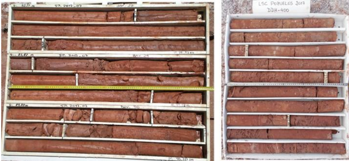
Figure 43: Lithologies from the HSU Mudflat (Source: WSP, Jan 2025)
