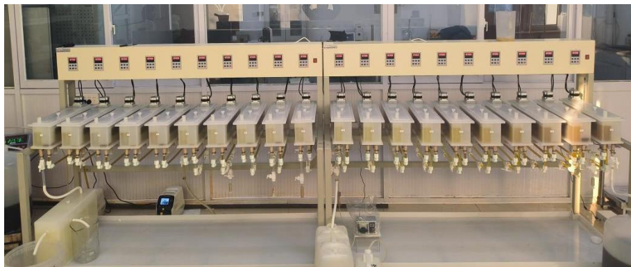
Figure 96: Continuous Extraction Device Diagram (Source: Ganfeng 2024)
