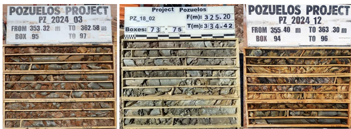
Figure 69: Photographs of the Fractured Aquifer (Source: WSP Golder, Jan 2025)
