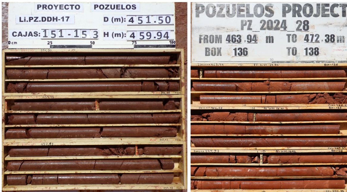
Figure 46: Lithologies of the HGU Siltstone (Source: WSP Golder, Jan 2025)
